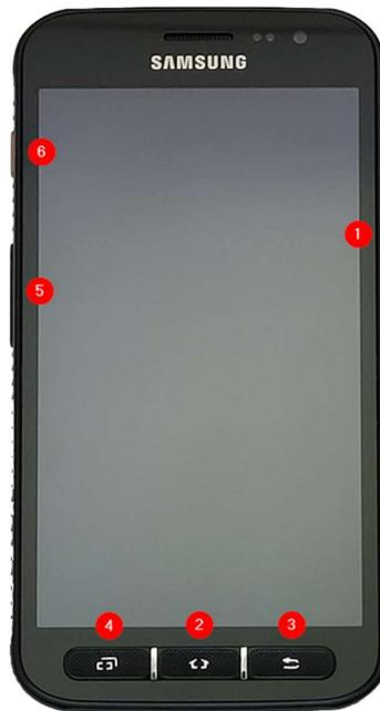
1. Power button - press and hold to turn the phone on / off
